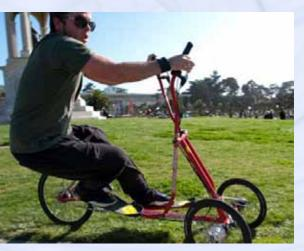
the motion of jogging, cycling and cross-country skiing into one. The elliptical motion of the feet drives the chain, while the arms push on the Strider poles, adding extra torque to the rear wheel. Steering is accomplished by
